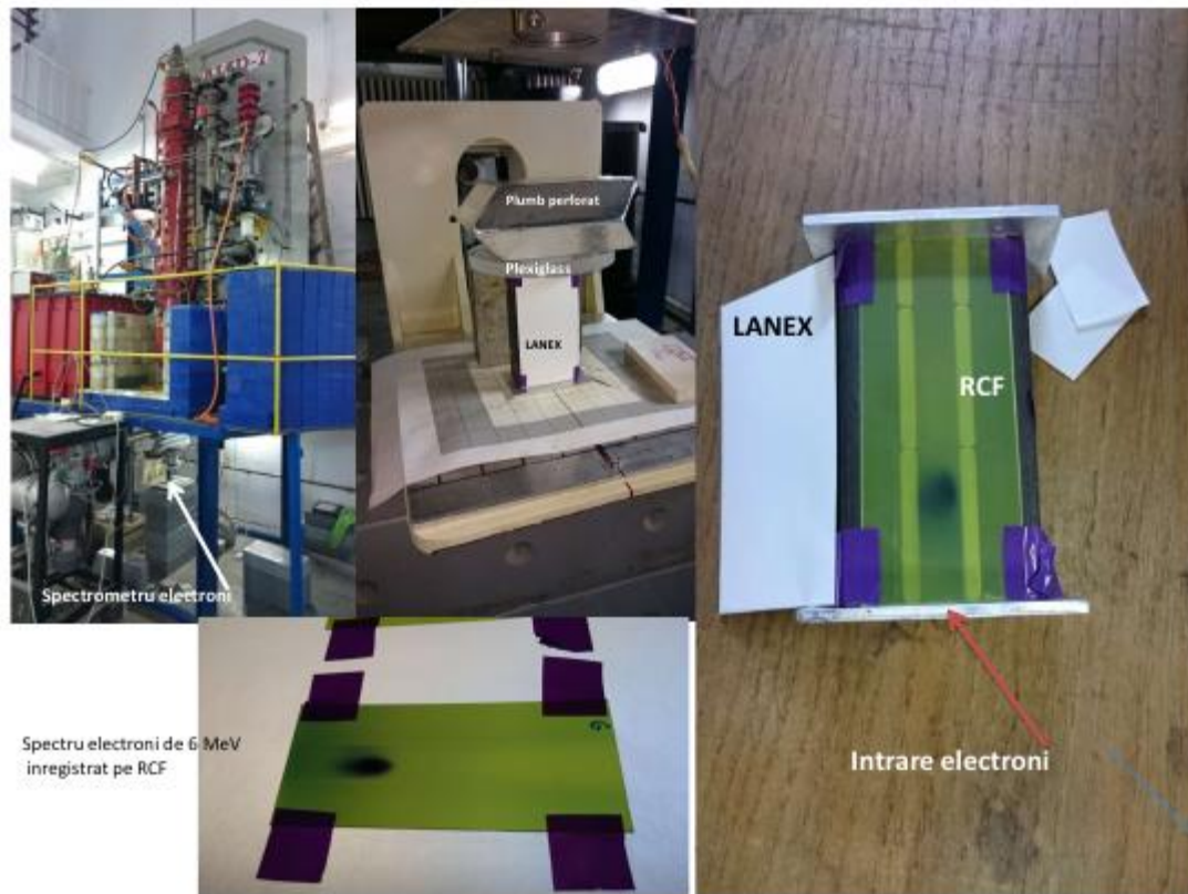
Figure 6: Electron spectrometer calibration using an accelerated 5.5 MeV energy electron beam and the classical accelerator ALID 7 from INFLPR
